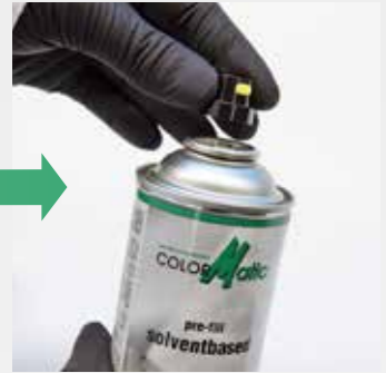
Remove the spray head
