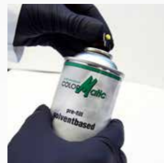
Replace the spray head
