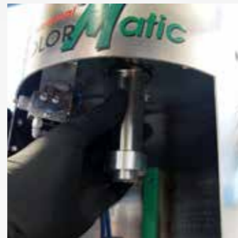
Fit the piston and piston rod
