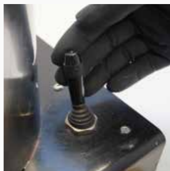
Pull the lever forwards. The can is now filled with the paint
