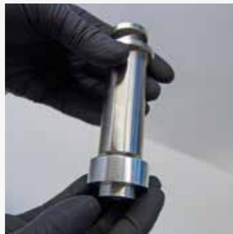
If required, replace the teflon piston with the metal piston
